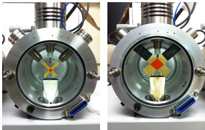
Figure 2. IonDrive™ Turbo V source. Optimized geometry and larger diameter heaters result in higher ionization efficiency and robustness.
